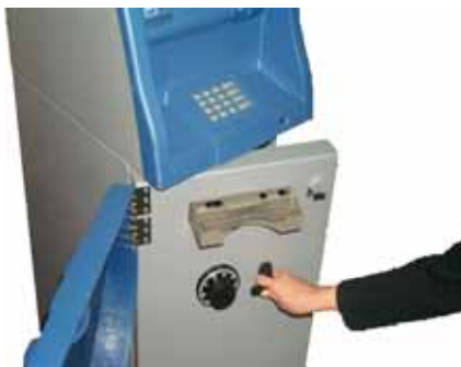
Fig.A-1 Opening the Security Door
